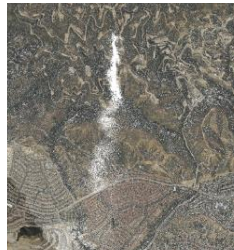
AVIRIS-C: 1/12/16 White pixels indicate plume detection
